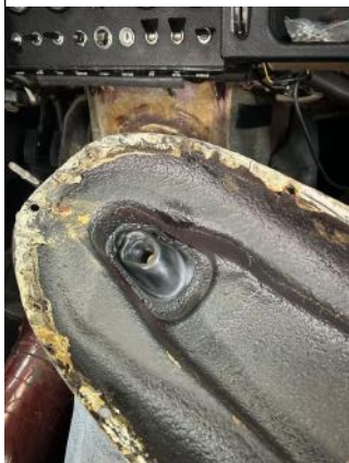
4—underside of transmission cover needs to be cleaned
