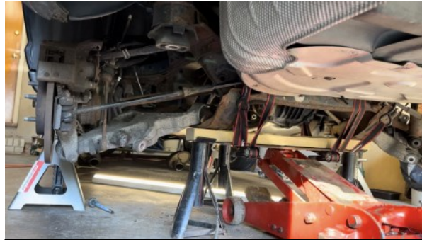
Dropping the rear suspension to gain access to the carbon canister.
