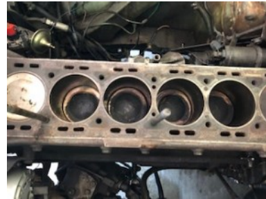
Condition of the pistons et al when head was removed.
