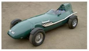
Power is supplied by a 6.0-liter Jaguar V-12 fed by six Weber downdraft carburetors making around 375 HP.
