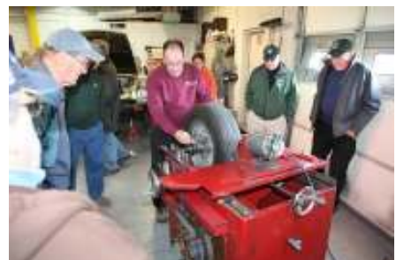
Ken Beck demonstrating the tire shaving machine and process.
